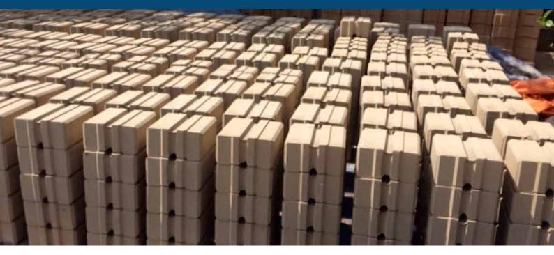
interlocked to the others, but is not bonded to the them as with cement mortared bricks. With traditional mortar, once there is a soil movement, the bricks come under such strong tension that the bond eventually cracks and the wall starts a cracking process that never ends and is most difficult to correct. With our Stabilised Earth Bricks, each brick undergoes a minimal amount of movement and the whole wall will adjust progressively without damage or cracking.
